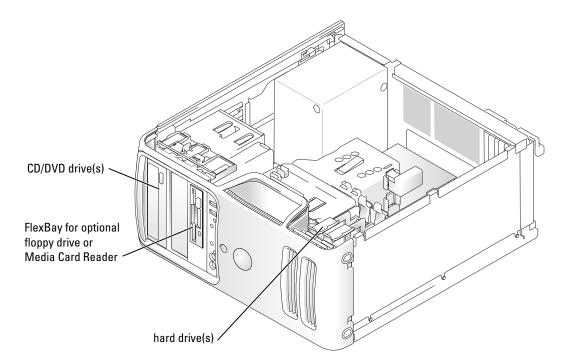
Connect CD/DVD drives to the connector labeled "IDE1" on the system board. Serial ATA hard drives should be connected to the connectors labeled "SATA0" or "SATA2" on the system board.
